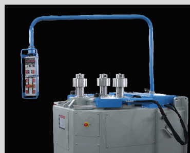
AR-41 with modified arbors, dies, and lengthened guide roll in/out travel
