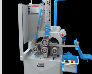
AR-14 - 4roll angle roll equipped with: high speed 80FPM drive, infeed guide for squaring parts, and light curtains.
